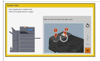
Two or more sheets of original are fed together. Remove the misfed originals and check their condition. Then replace them on the ADF. For details, see the reference below: P.16 "ADF"
