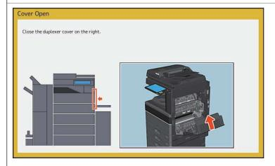
A cover is open. Check which cover on the touch panel and then close it securely.
